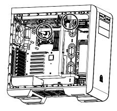
onnect the tubing and check all the fittings are sealed. The loop order: Water black > Reservoir Inlet
