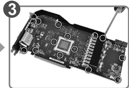
Remove the bracket (Remove encircled screws on the bracket)
