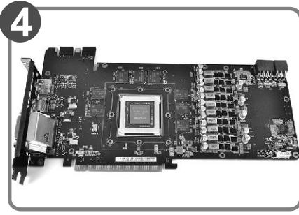
Clean the original thermal compound off the GPU die. (Carefully detach the original stock cooler after removing all screws securing the cooler to the board)
