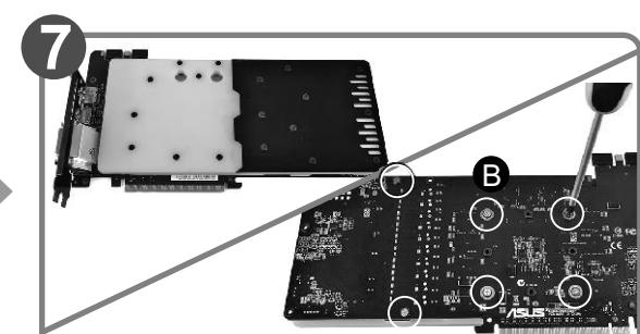
When installing the water block, carefully position the water block with the preinstalled standoffs on the graphics card.
