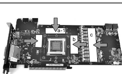
Cut the thermal pads to the dimensions listed and place them on the spots shown on the diagram.
