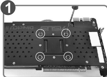
Remove original VGA stock cooler (Remove the screws circled on the diagram. All heat sink assembly screws should be removed)
